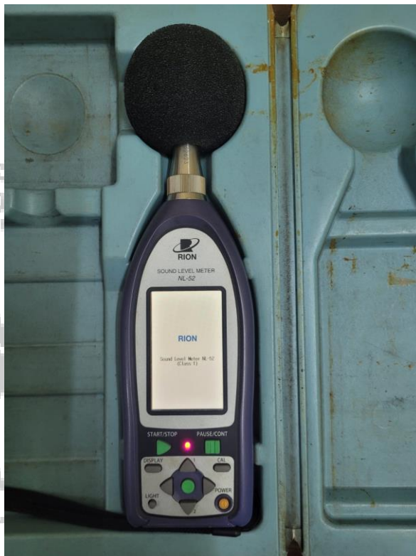
Figure 15. Noise Meter used for measurement
